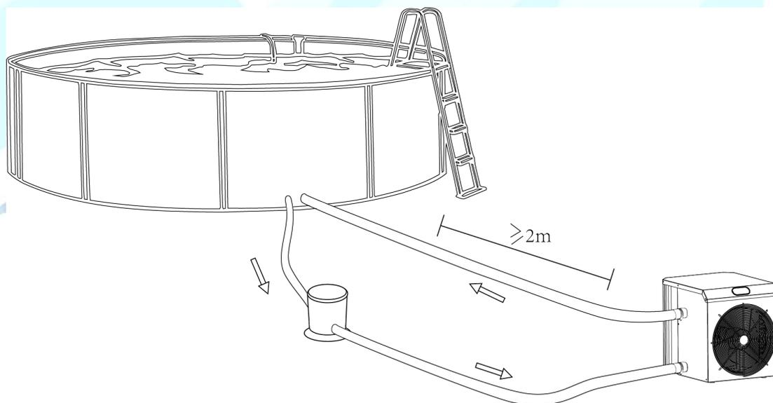
**Attention!** Do not install the unit in a confined or insufficiently ventilated location, or in a place where it may block the air intake. These locations can affect the air flow, it will cause the air to recirculate, resulting in reduced efficiency. It even may stop the system from running.
